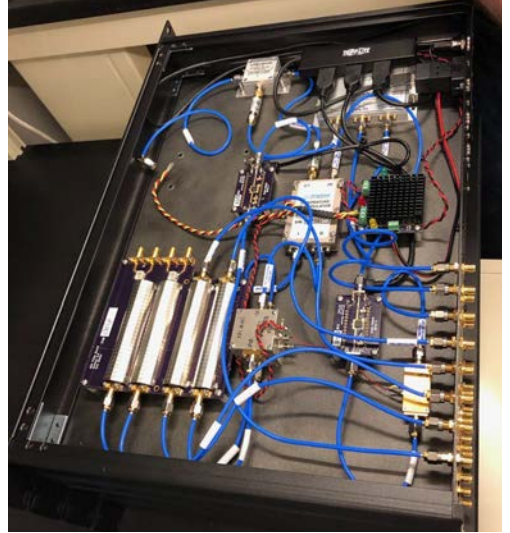
Above: RF/IF components for interfacing with ROACH-2
